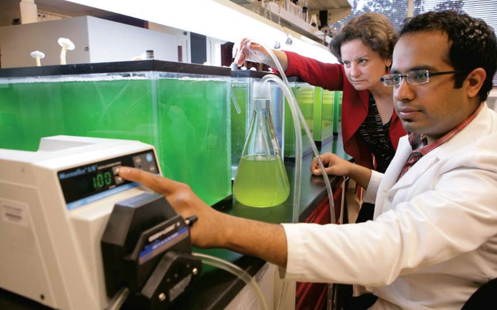
Dr. Barbara Benson, assistant professor of environmental science, and chemical engineering graduate student Harry Daultani inoculate a bioreactor tank with algae.
