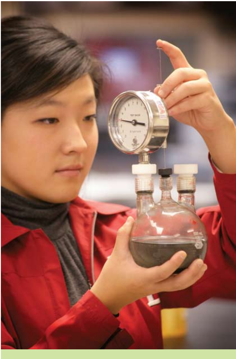
Chemical engineering student Bridget Meaux measures the amount of methane being produced by fermenting sewage sludge.
